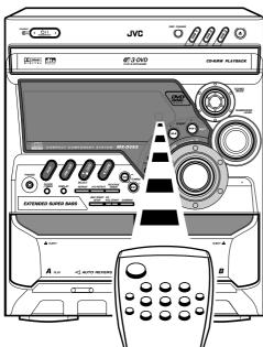
When using the remote control, point it at the remote sensor on the front panel.
